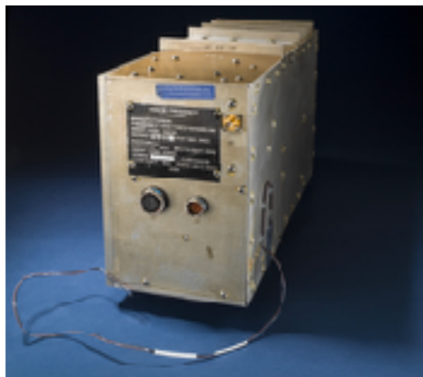
Cs atomic clock built for the first GPS satellites (late 1970s)
