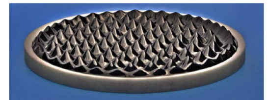
Figure 1. The Rosensweig instability [32] of a ferrofluid (a colloidal dispersion in a carrier liquid of subdomain ferromagnetic particles, with typical dimensions of 10 nm) in a magnetic field perpendicular to its surface is a fascinating example of the novel physical phenomena appearing in classical physics due to long range, anisotropic interactions. Figure reprinted with permission from [34]. Copyright 2007 by the American Physical Society.
