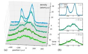
FIG. 3. (i) Longitudinal expansion of a cloud of  $N = 6300 \pm 200$  atoms initially trapped in a double-well potential, compared with GHD. (ii) Even though the initial state is the same for GHD and CHD, both theories clearly differ at later times. CHD wrongly predicts the formation of two large density waves. The error bar shown at the center at t = 40 ms corresponds to a 68% confidence interval, and is representative for all data sets.
