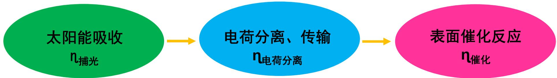
$$\text{太阳能转化效率 } \eta = \eta_{\text{捕光}} \times \eta_{\text{电荷分离}} \times \eta_{\text{催化}}$$
